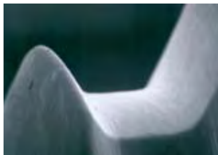
Optimised surface of a Guhring form tap
