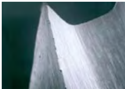
Surface of a conventional form tap
